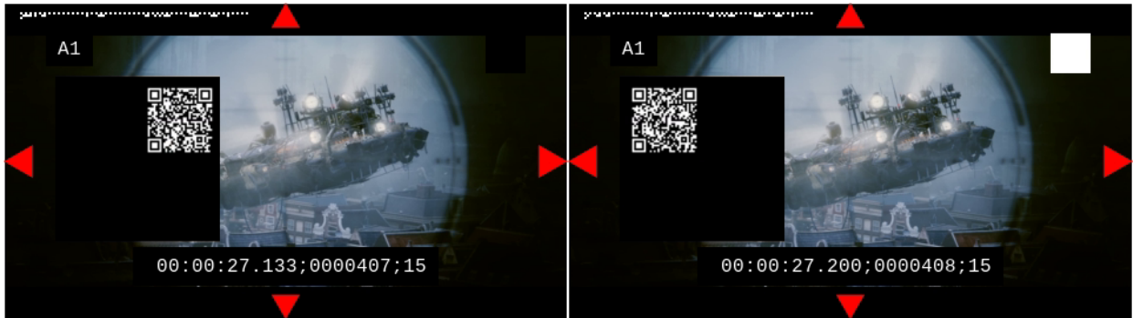
Figure 12: Examples of the audio sync mark indication in the absence of audio feedback (left) and during audio feedback (right)
